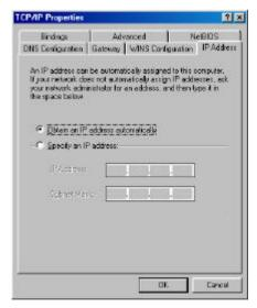
Figure 3: TCP/IP Properties
